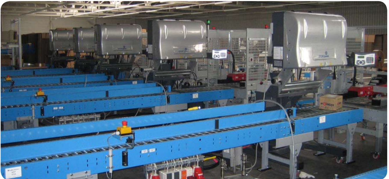
Multiple FOAMplus® Bagpacker machines integrated in a direct conveyor technique.
