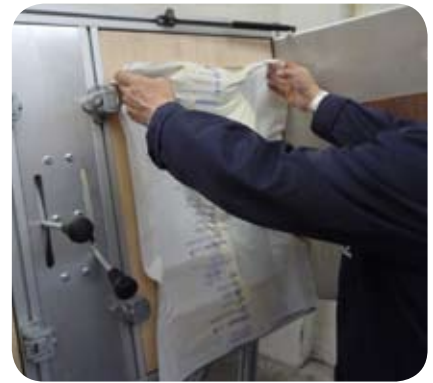
Step 2: The operator places the foam-filled bag in the wooden mold.
