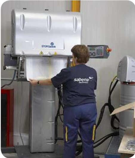
FOAMplus® Bagpacker machine with a single packing table solution.
