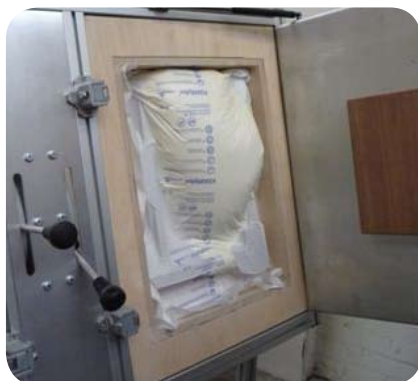
Step 3: The mold is closed to allow the foam to expand inside.
